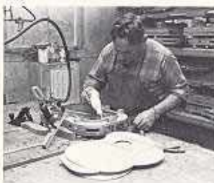
Top Sound-board and Back are glued to the sides.
