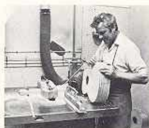
The channel for inlays and binding are cut out with specialist tools.
