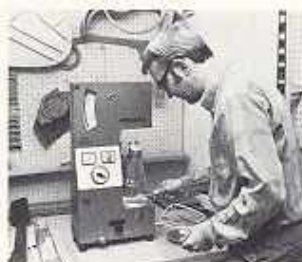
During the entire manufacturing process the degree of moisture in the wood is kept under close observation.
