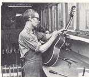
Fitting the guitar's neck is one of the most important manufacturing steps
