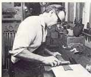
The fretboard receives some fine adjustment before final assembly
